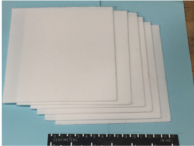
Figure 4.7: Six Layers of Alumina Paper Insulation
